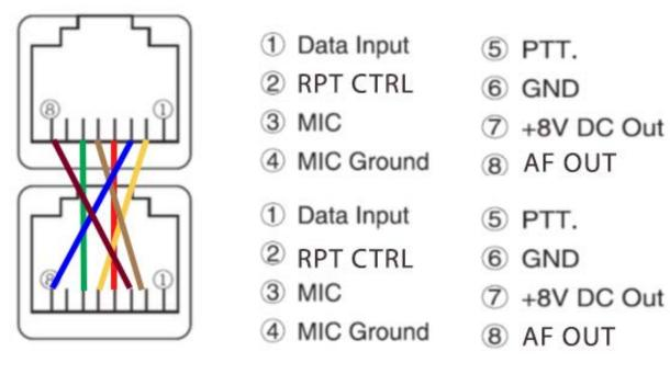
WIRE PINS: 2 TO 5, 3 TO 8, 4 TO 4, 5 TO 2, 6 TO 6, 8 TO 3
