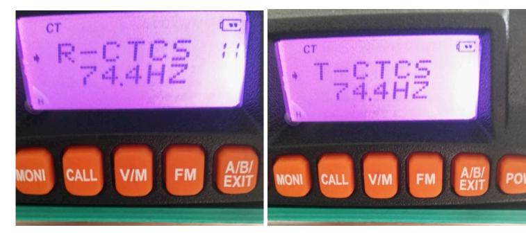
3: Enter MENU 43 REP-M and select CTDCS for two mobiles – this will require the repeater forwarding (X-Band Repeat) to activate once the confirmed PL signal (CTCSS or DCS) is received will transmit it on.
